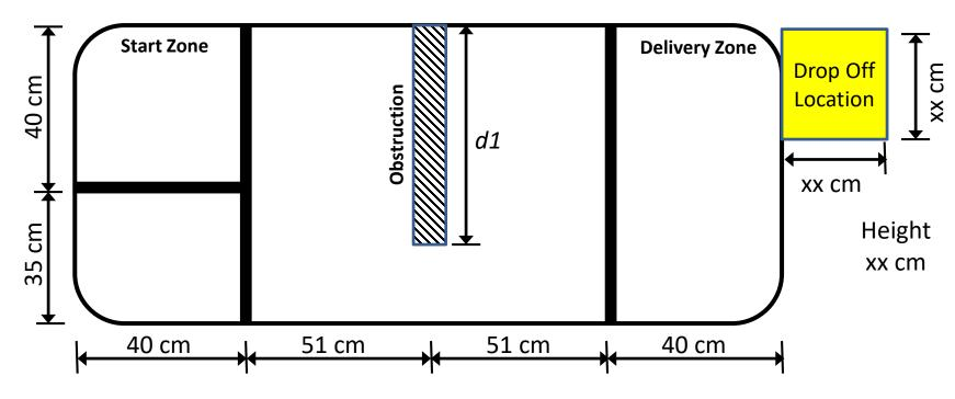
Your robot must begin in the Start Zone and deliver a ping pong ball to the Drop Off Location (cardboard box). After the ball is delivered, your robot must return to the Start Zone. Once the robot completely reenters the Start Zone, you may reload your robot with another ping pong ball and deliver the ball to the Drop Off Location. You are awarded points based on the number of ping pong balls successfully delivered to the Drop Off Location.
